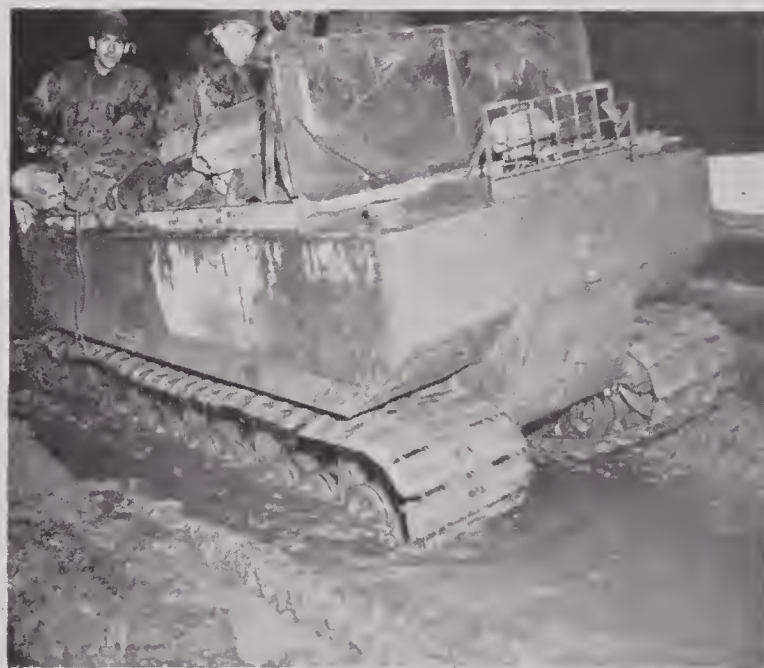
FIGURE 65. A flooded road in Germany provides sufficient traction for an M-29 Weasel.
